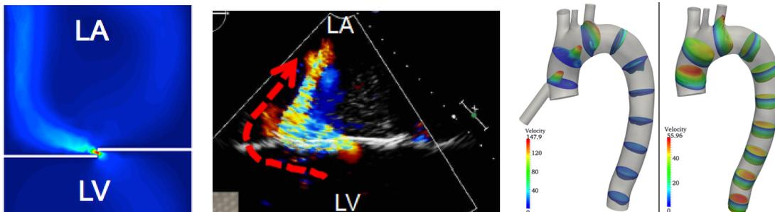
Left and center: computational simulation (left) and in-vitro reproduction (center) of a mitral regurgitant jet from the left ventricle (LV) into the left atrium (LA). Right: computed blood velocity in a human aorta when blood is pumped from the LVAD (left) and it is pumped from the heart (right).
